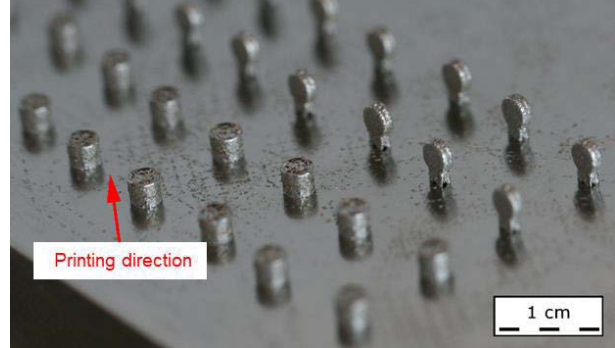
Figure 3: \varnothing 3 \text{ mm} NiTi-disks on SLM-building platform in horizontal (along cylinder axis) and vertical (in radial) printing direction.
